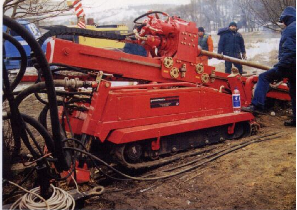
This Powermole/SE PM903 dry rock drilling system was used on projects in the Czech Republic and in Scotland.
